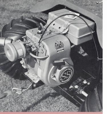
Check this power plant, a Tecumseh 4-cycle 5-horse frisky that'll purr or roar to your mood. Top speed is a sparky 25 mph, and that tank holds 2 gallons . . . enough for a long romp! The body's molded fiberglass, frame's 2-inch tubular steel.
