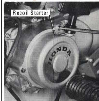
STEP 24 - Reinstall starter pulley and recoil starter.
