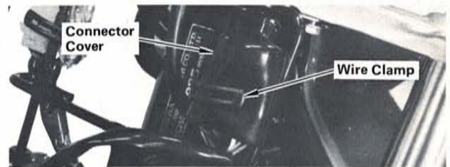
STEP 39 —Open wire clamp holding connector cover and turn cover inside out as shown. Connect headlight wire harness connector to black connector and pull connector cover over connectors. Secure connector cover with wire clamp as shown.
