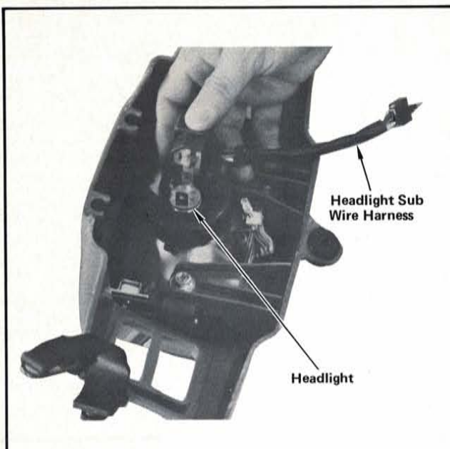
STEP 38 —Connect headlight sub wire harness to headlight as shown.
