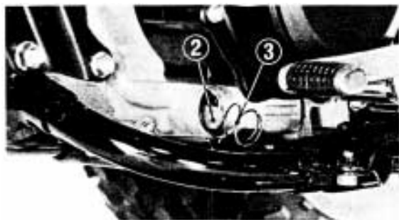
(2) Oil filter screen (3) Spring
