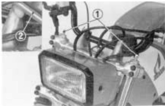
(1) Air valve caps (2) Pressure gauge
