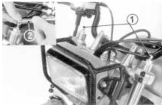
(1) Air valve caps (2) Pressure gauge
