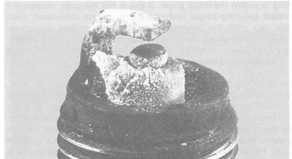
White deposits have accumulated from excessive amounts of oil in the combustion chamber or through the use of low quality oil. Remove deposits or a hot spot may form
