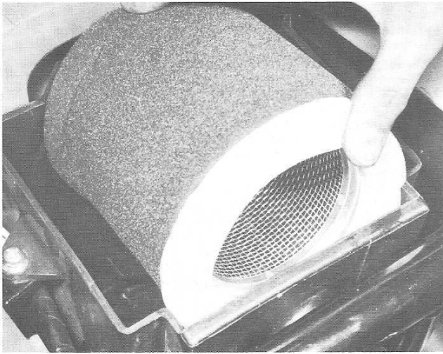
5.3 ... to expose air filter element – note element supporting frame
