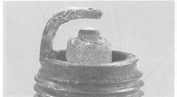
A worn spark plug not only wastes fuel but also overloads the whole ignition system because the increased gap requires higher voltage to initiate the spark. This condition can also affect air pollution
