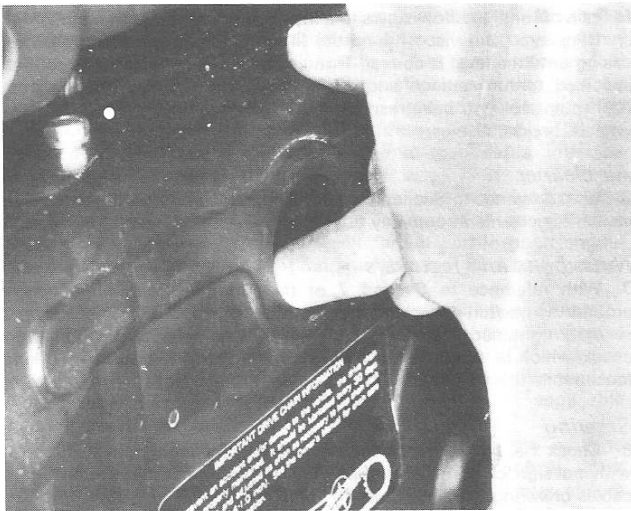
3.4a Checking drive chain free play – measure at tightest point in chain run
