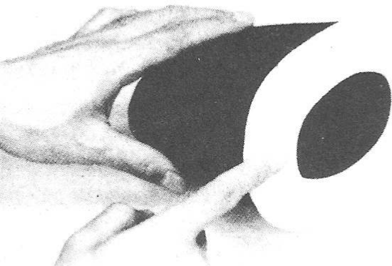
Fig. 1.22 Apply grease to the end(s) of the element to ensure sealing in the airbox (Sec 13)
