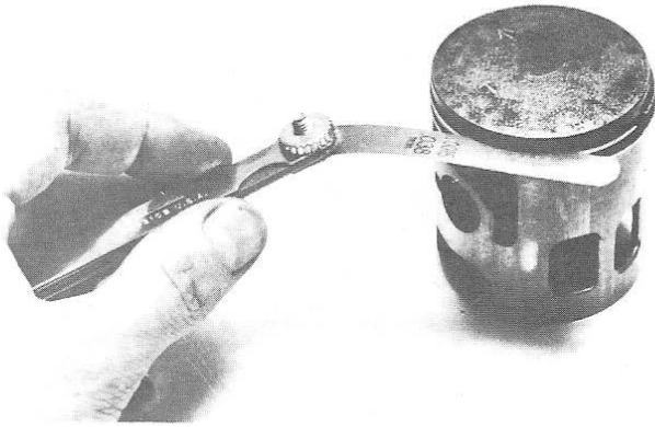
9.13 Checking the piston ring-to-groove clearance (move the feeler gauge around the piston and make the check at several points)
