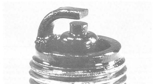
Wet, oily carbon deposits form an electrical leakage path along the insulator nose, resulting in a misfire. The cause may be a badly worn engine or a malfunctioning ignition system
