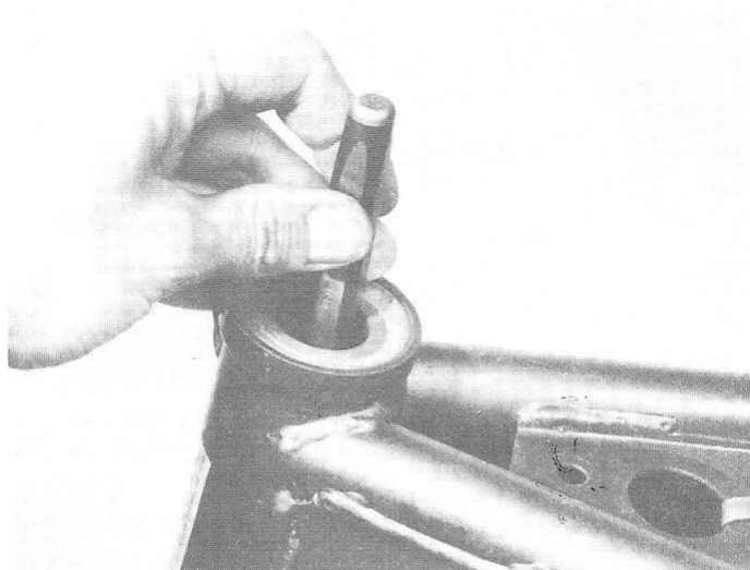
6.8 Position the punch against the back side of the lower race and tap it with a hammer to drive out the race
