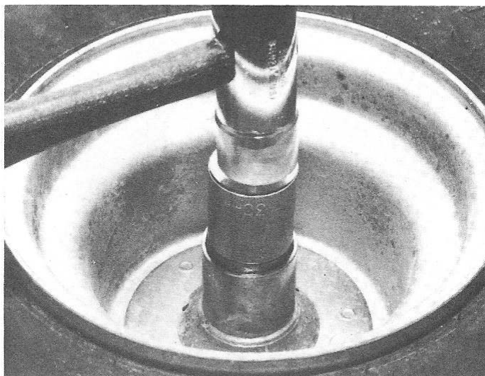
18.17a Installing a front wheel bearing with a hammer and socket
