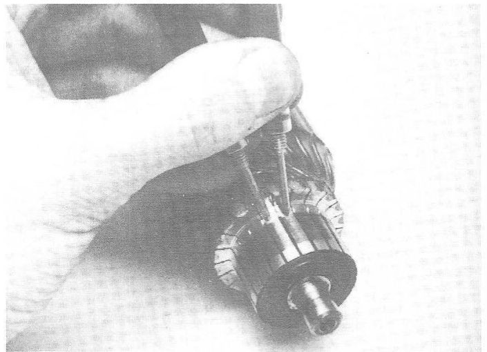
16.9 Checking for continuity between the commutator bars
