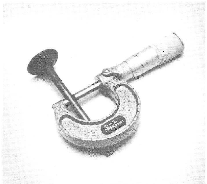
9.18 Measuring the valve stem diameter with a micrometer
