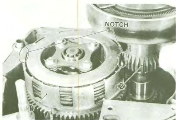
1. Clutch housing 2. Primary drive gear
