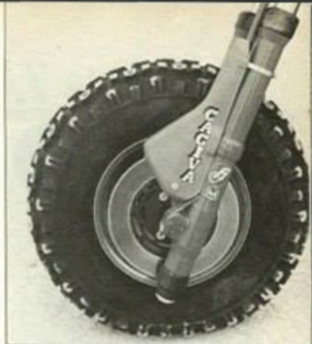
40mm front forks offer 9.75-in. of travel and, although a little on the soft side, worked great in the rough. Front disc brake also worked very well.
