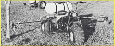
This self-contained MICRON BOOM SPRAY SYSTEM features an 11 gallon Poly tank and 12 volt electric fluid pump. The Controlled Droplet Applicator (CDA) nozzles produce uniform micron sized droplets. Boom sizes range from 3'-10' with adjustable heights of 8"-20". The booms articulate to prevent damage to the heads.
