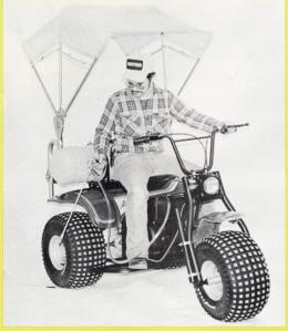
This AVENGER 300 is shown with a canvas "buggy top" CANOPY which can be easily adjusted to shade the driver. The self-contained SPOT SPRAYING SYSTEM uses an 11 gallon Poly tank, 12 volt electric fluid pump, and an 18" hand operated wand with an adjustable tip.
