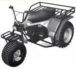
This AVENGER Big Foot is equipped with a carryall MAGNUM CARGO RACK. The FRONT RACK attaches easily to the front fork for extra carrying capacity.
