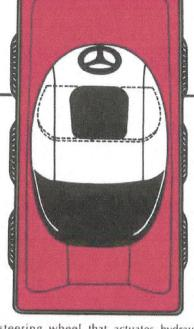
plished by a steering wheel that actuates hydraulically controlled disc clutches. Moving the wheel to the right disengages, then brakes all three right wheels while the left wheels power... and vice versa.
