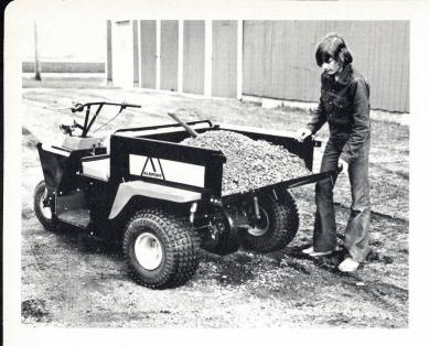
The **UT-10 Dump Truck** is quiet . . . and it is smooth. It is fully suspended at each wheel with hydraulically dampened shocks assisted by coil springs. All shocks are fully adjustable for ride control.
