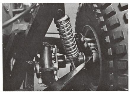
Rear suspension: "A"-frame with dual shock absorbers.
