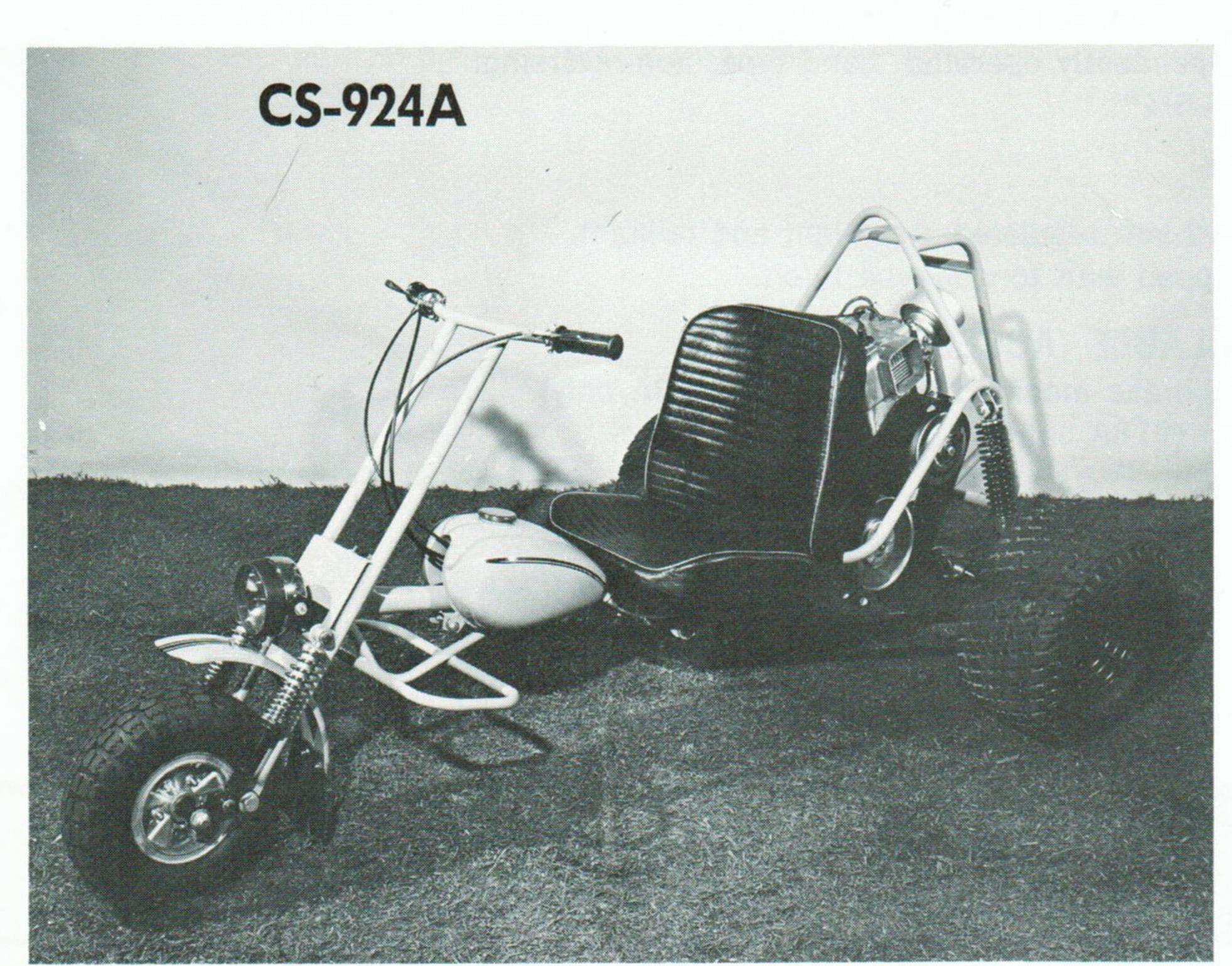
And here's all the horsepower you need to horse around. All of the features above PLUS a 290 cc - 2 cyl. - 24 hp. Kohler engine. Ride in comfort and safety surrounded by a heavy duty tubular frame with roll cage and frame mounted gas tank. With independent front and rear suspension, it handles like a dream at speeds up to 55 mph.
