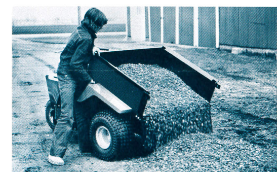
Dump Bed Holds 1/4 Ton. Over Center Bed for Easy Emptying
