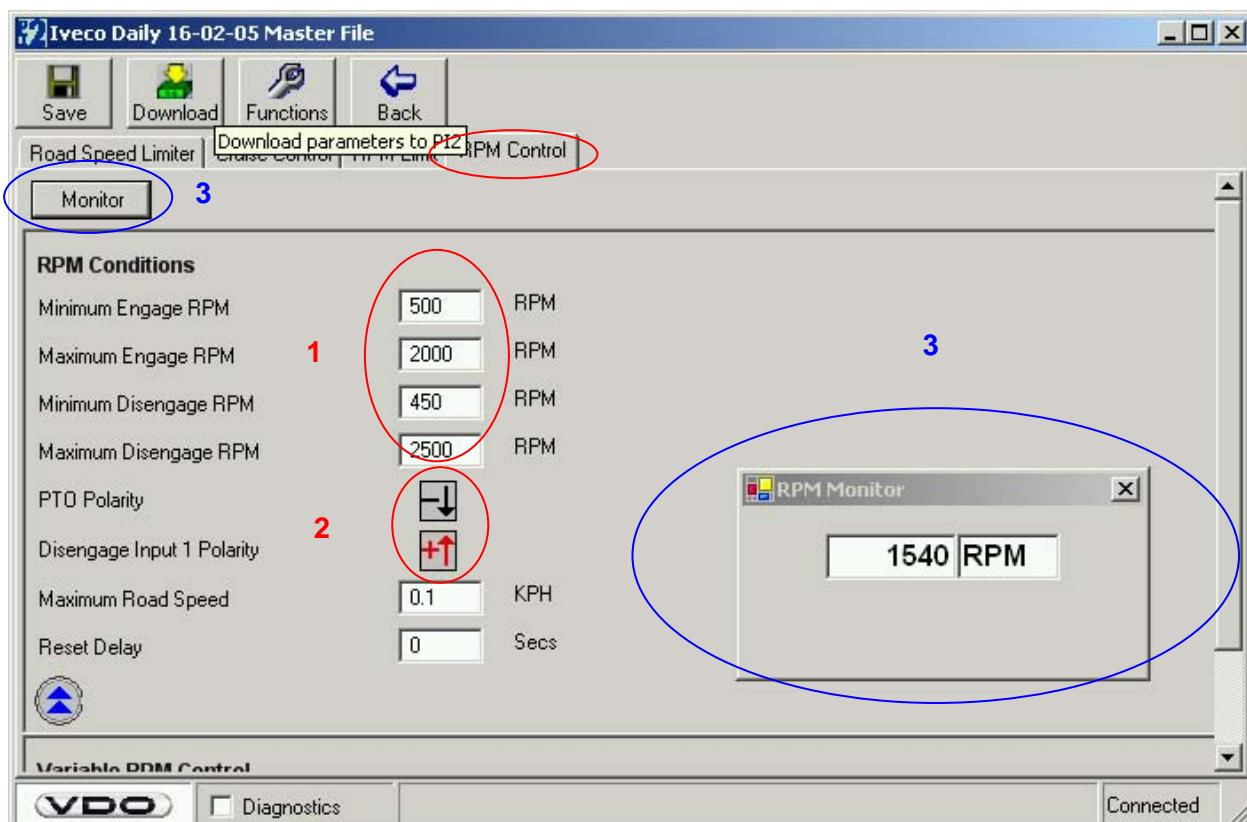
1 → Input the min, max engage and disengage of rpm control.
