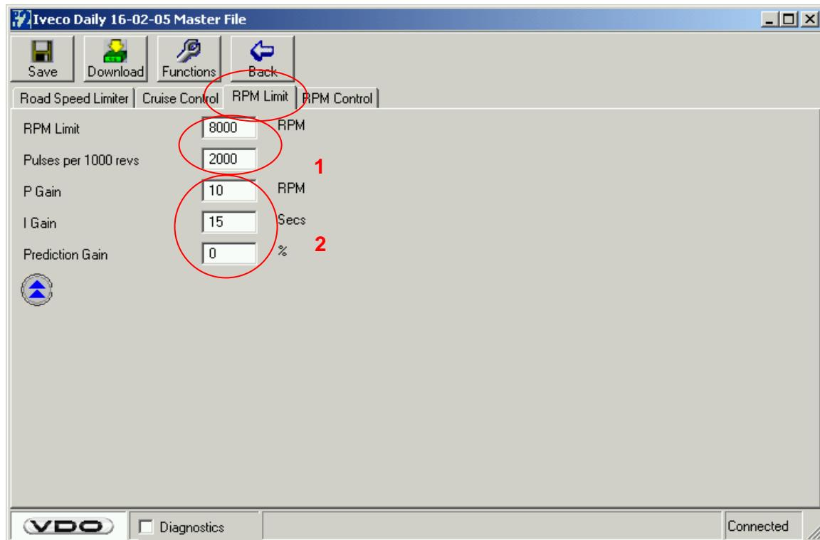
**1 →** Input of desired engine speed limit and the vehicle-specific engine speed pulses. If the engine speed limitation is not in use, 8000 rpm should be entered as the limit.
