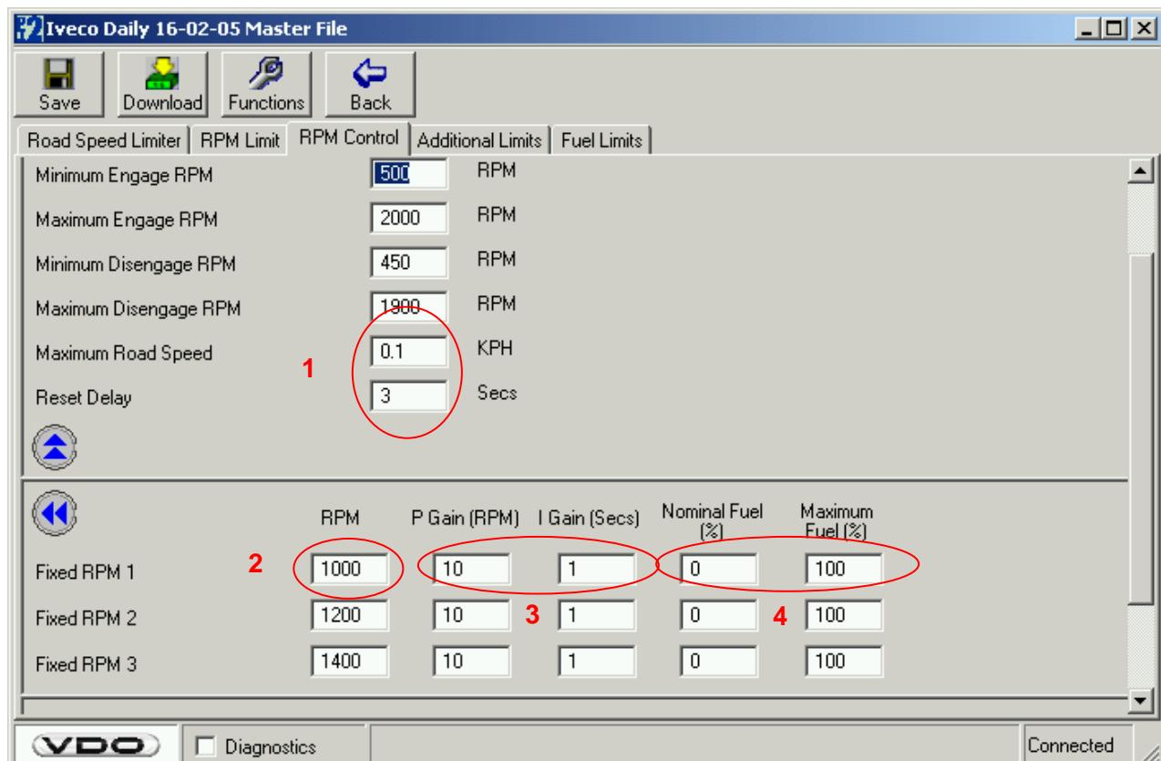
**1 → Maximum Road Speed** – Allows an additional disengage function of the rpm control when the road speed exceeds the speed set in this window.
