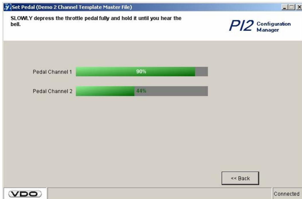
Wait until for the audible alarm or follow the instructions in the page heading. Slowly release the pedal. After a successful throttle pedal setting, the configuration manager will automatically download new data and open the function select page.
