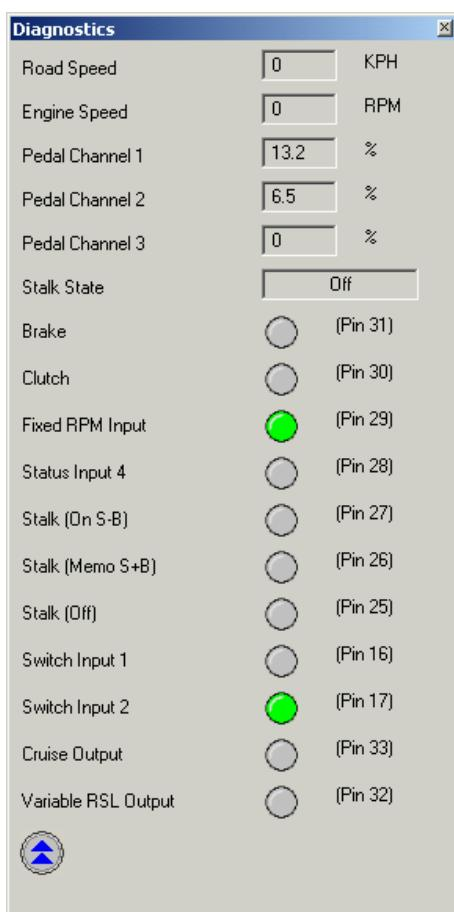
In the diagnostics window engine speed, road speed signal and pedal values are displayed
