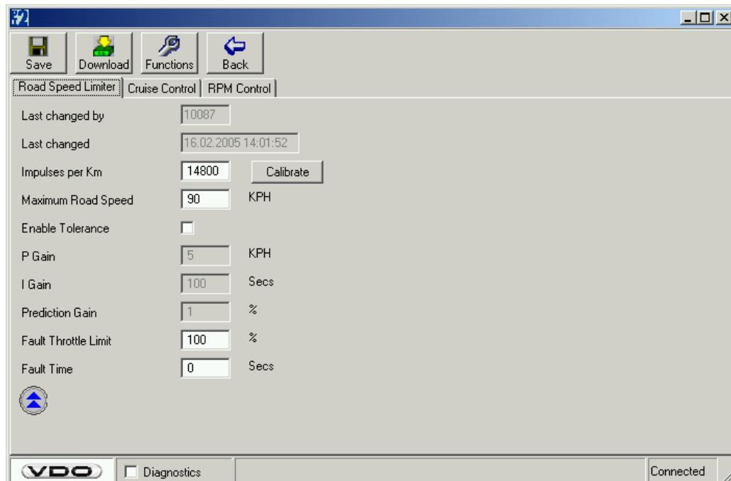
1 → If the pulses are known, it can be programmed directly to this Window. If not a calibration function is possible.
