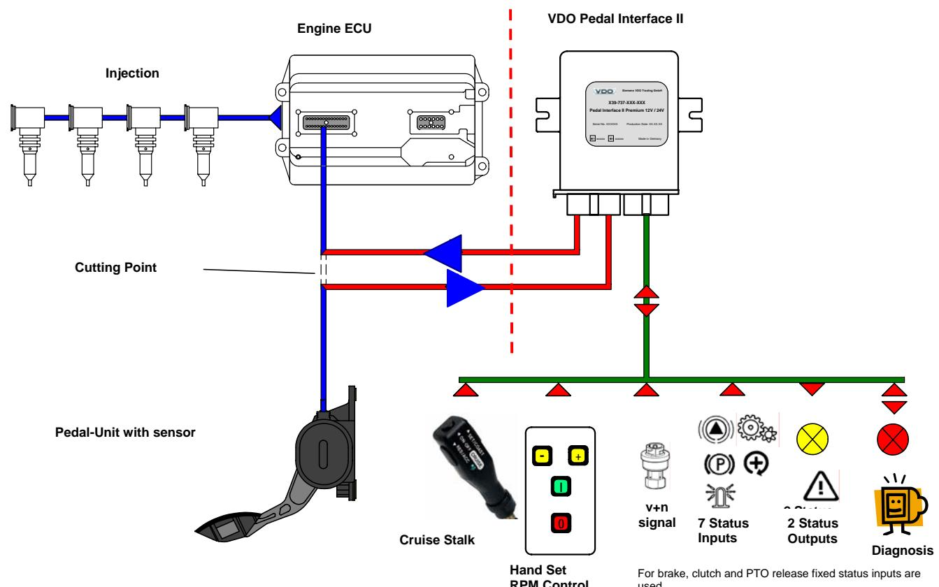
The vehicle accelerator pedal is displayed on the left side; the engine control unit and the fuel injection are part of the existing vehicle system. The Pedal Interface II with all inputs and outputs, displayed at the right side, are installed additionally into the vehicle and connected via the pre-manufactured wiring harness.
