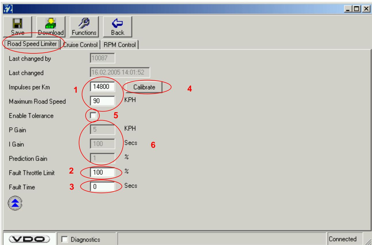
1 → Input of road speed pulses and maximum road speed.
