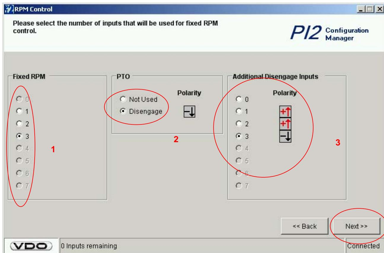
1 → - Number of fixed engine speed inputs (only positive polarity allowed)
