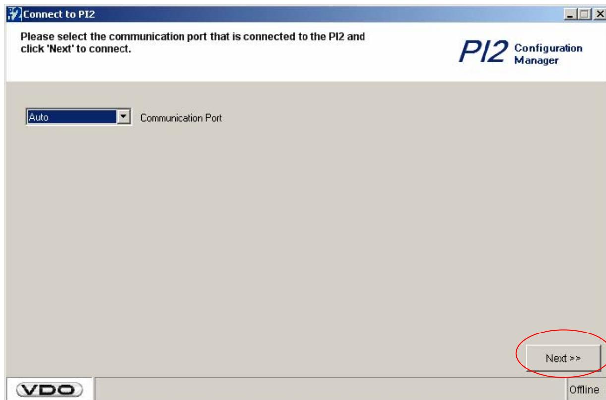
Once the Configuration Manager has connected to the VDO PI 2 control unit the Pedal Interface has now to be downloaded with the vehicle-specific data.
