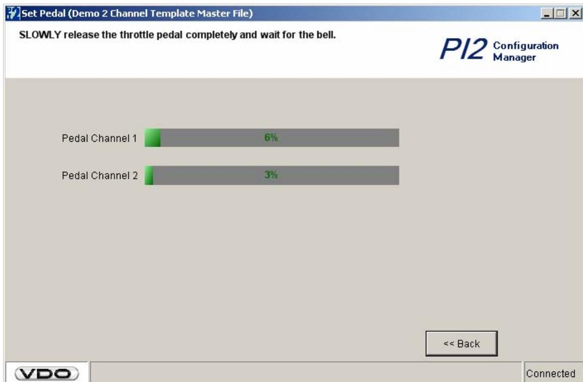
After a successful throttle pedal setting, the configuration manager will automatically download new data and open the function select page.
