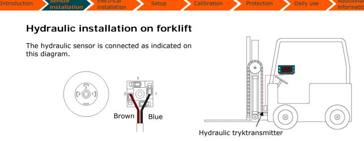
The hydraulic transmitter should be placed as close to the lifting cylinder as possible to obtain the best messuring accuracy.
