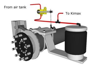
The pressure in the suspension system and in the bellows represents the weight of the vehicle.
