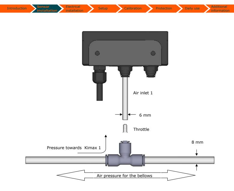
All air-inlets on Kimax instruments and all fittings are quick-release type.
