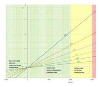
The gain is set by SCU in 6 steps. The output from the unloaded axle is recommended set to 15% of max signal.
