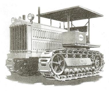
Motor—Six cylinder, four cycle, water-cooled, valve-in-head. Cylinders cast in pairs, 6 inch bore, 7 inch stroke. Crankshaft is of S.A.E. 1045 steel heat-treated, supported on four bronze-back, babbitt-lined main bearings which are 3¾ inches in diameter. Pistons are cast iron having four ¼ inch wide piston rings. Connecting rods are I-beam, drop forged, of S.A.E. 1035 steel, heat-treated.
