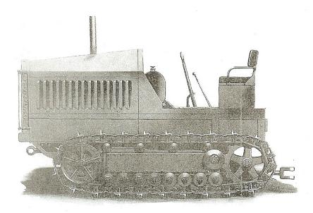
MOTOR—Six cylinder, four cycle, water-cooled, valve-in-head. Cylinders cast in pairs.  $5\frac{1}{2}$  inch bore,  $6\frac{1}{2}$  inch stroke. Crankshaft is S.A.E. 1045 steel, heat-treated, supported in four bronze-back, babbitt-lined main bearings which are  $3\frac{1}{2}$  inches in diameter. Pistons are cast iron having four  $\frac{1}{4}$  inch wide compression rings with one oil wiping ring. Connecting rods are I-beam, drop forged, S.A.E. 1035 steel, heat-treated.
