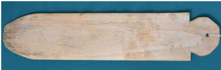
Photo 2: Wooden sock mold. The woolen socks are pulled over it to have them smooth.
