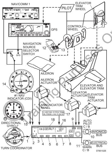
Figure 1. Bendix/King KAP 140 2 Axis Autopilot Schematic (Serials 17280831 thru 17281173) (Sheet 1 of 2)
