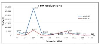
This ISCO project highlighted the importance of establishment of adequately located monitoring wells within the radius of influence. The San Diego RWQCB issued a Closure of the Site (No Further Action) in late 2013.
