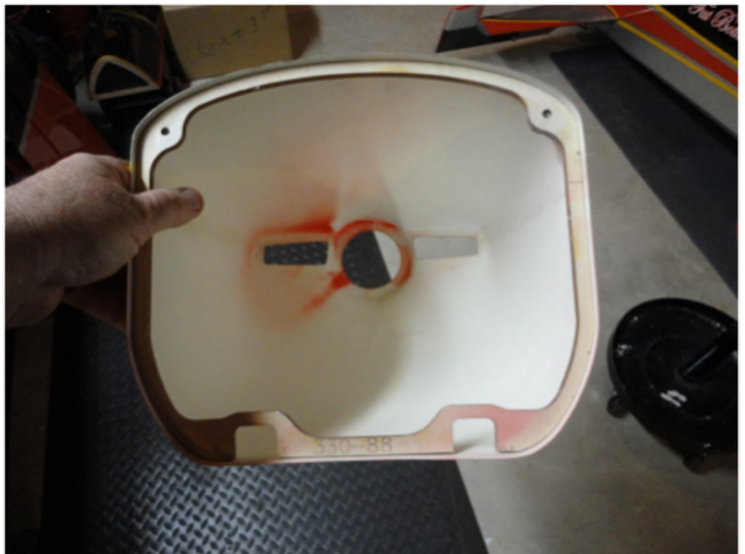
The turtle deck is typical foam that is balsa sheeted. The underside of the fuse has a canister tunnel built in.
