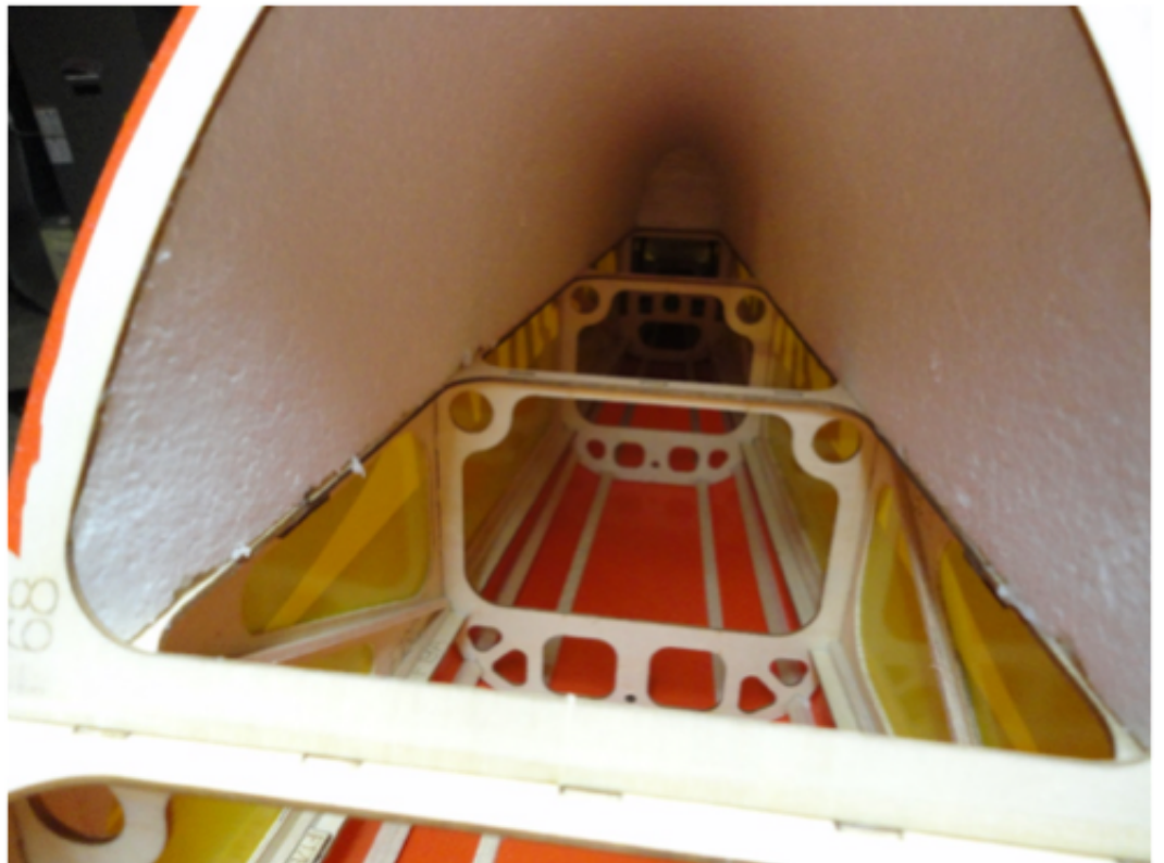
The turtle deck is typical foam that is balsa sheeted. The underside of the fuse has a canister tunnel built in.
