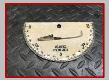
out and glued it to a piece of plywood and drilled a hole in the base so it can be slid onto the crankshaft and you're in business. You will also need some kind of pointer to let you know where you're looking at the timing mark. I made mine from a piece of wire soldered onto an alligator clip so it will attach to the cylinder fins.
