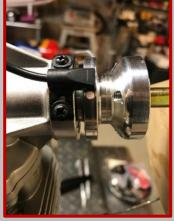
adjustment, and move the Hall Sensor in the same direction as normal rotation to retard the timing. If it is firing late or retarded, it should be moved in the opposite rotation to the advance timing.
