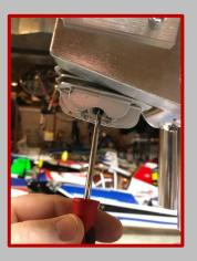
2) Or, with a small screw driver put it in the spark plug hole while bringing the piston all the way up to TDC slightly rotating the crankshaft back and forth finding the point at which the
