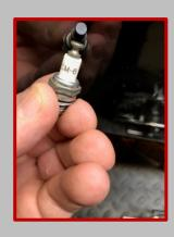
Some of the other pictures are of proper plug to cap seating and other components of a typical capacitive discharge ignition system. As much as I like DLE engines, the spark plugs that come with them are guaranteed to fail prematurely. Replace them with an NGK CM-6 or Nippon Denso plugs. Always make sure your wiring is tied down to something, i.e. Zip-Ties or sticky back hold downs.
