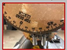
several times to find the exact point at which it fires. A properly set timing should be around 28-30 degrees before TDC. If it fires at 35 degrees, or higher, it is too far advanced. Loosen the screws holding the Hall Sensor, (nothing more than a magnetic on-off switch) which has slots for
