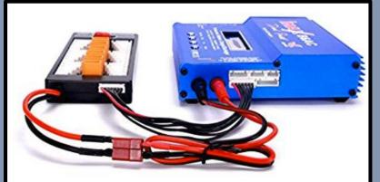
Example: Single Port battery charger with a 6 Port XT-60 Parallel Balance Port Charging board connected. Batteries will connect to the Parallel Charging Board.
