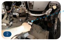
This is a vehicle OBDII connector.
