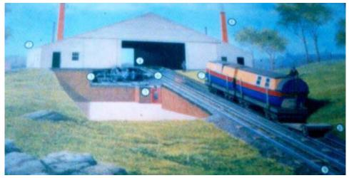
As you approach the hoist house along a short interpretive trail from the visitors center, this sign shows how the inclines worked. The cars approaching the hoist house carry sectional canal boats, which could be broken apart for carrying over the Portage. This eliminated the timeconsuming practice of transferring between boats and rail cars. Relatively few of these sectional canal boats were built, however, and they came too late to make a difference. This, and the high maintenance costs of
