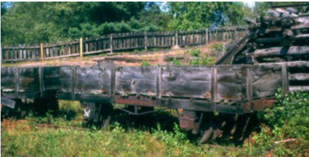
In the 1870s, when the half-mythical Molly Maguires terrorized non-Irish folk in the Anthracite Region, the Reading Coal & Iron Company and its parent Reading Railroad hauled coal to market in 4-wheeled cars called “Jimmies.” This is one of a short string of replica “Jimmies” spotted under the tippie at the Eckley breaker. It is a reasonable facsimile of cars actually used by the Reading Co. and matches the cars in the coal train blown up in the movie by the characters played by Connery and Harris.
