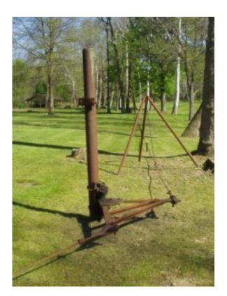
The pictures at left and below illustrate the complex system of connecting rods and linkages that allowed a single engine to power several pumps.
