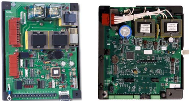
Group 1 Controller (left), Group G Controller(right) with covers removed
