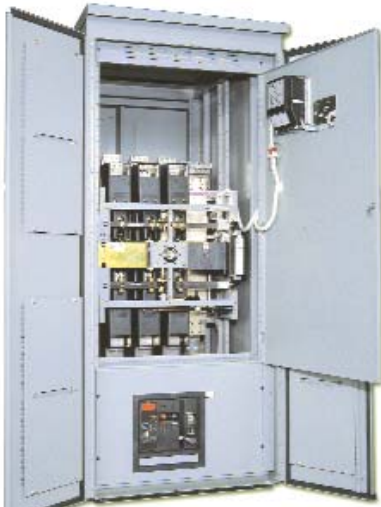
Fig. 15: ASCO Service Entrance Power Transfer Switch rated 3 Pole 2000 amperes shown in Type 3R secured double door enclosure with solid neutral
