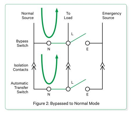
3. Allows the transfer switch to be electrically tested and operated without interrupting power to the load. With the bypass-isolation mechanism in Test mode, the transfer switch is disconnected from both power sources and the load and the normal bypass contacts carry the full load, as shown in Figure 3. The transfer switch operating circuits remain connected to the controls through secondary disconnects to allow electrical operation testing without interrupting the load.
