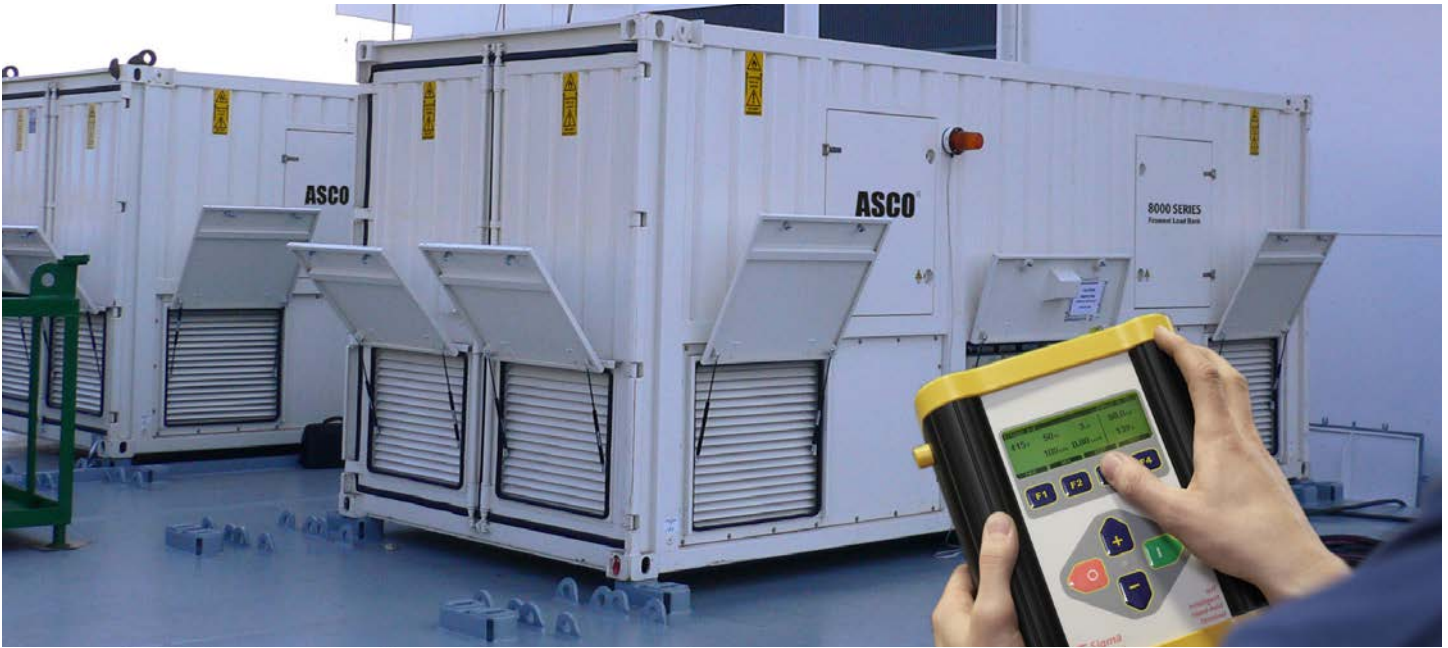
Two 6 MVA containerized load banks networked together.
