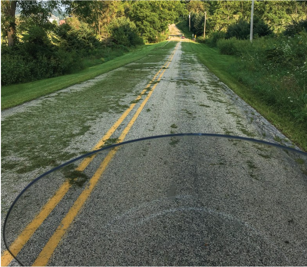
Grass on the roadway can be a non-issue or an extremely slippery condition. If possible, slow down using clear pavement ahead of the covered area.
