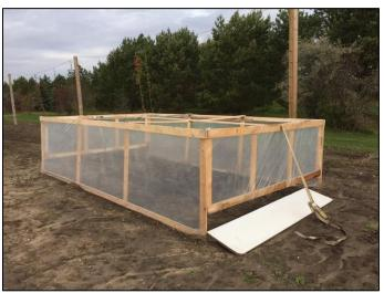
Figure 2. Rectangular heat chamber test design – built to span three potato rows and installed and removed multiple times in season.
