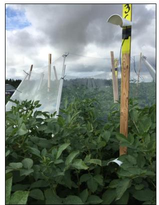
**Figure 1.** Hexagonal Plexiglas heat chamber design installed in a potato plot. Themocouple sensors installed on stakes inside and outside the chambers to monitor canopy temperatures.
