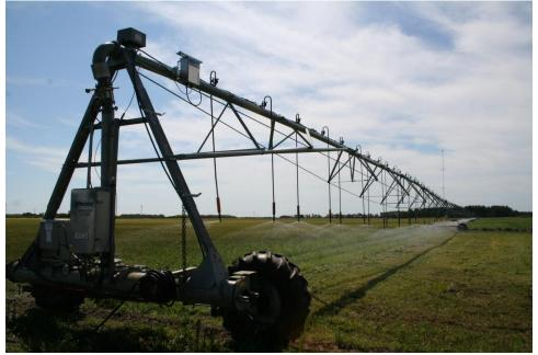
Figure 1. Lateral move irrigator with upgrade to Variable Rate Technology.
