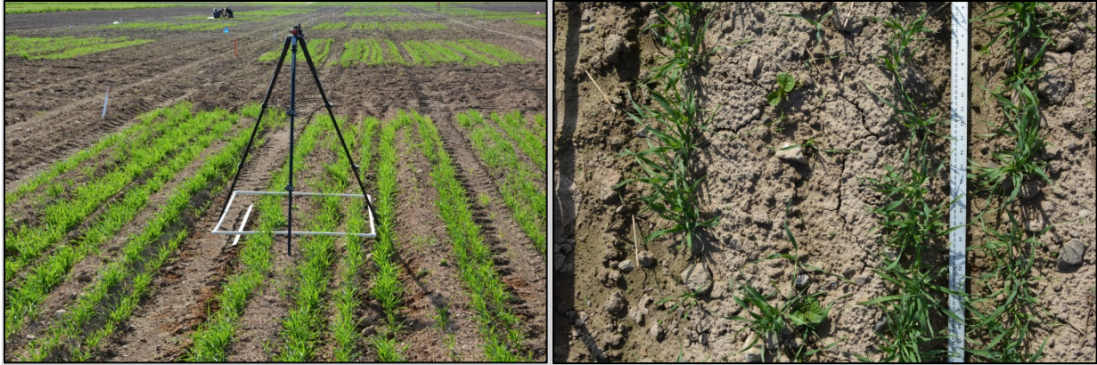
Tripod set-up used to capture aerial picture of nurse crop (left); and resulting image used to quantify soil cover (right).
