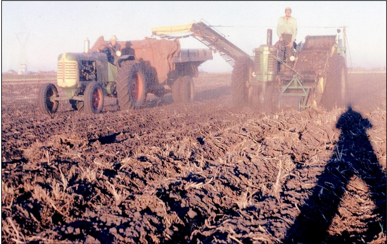
Fig 1. Potato harvest in Carberry, Manitoba in the mid-1960s. Several items are particularly interesting about this photograph. For example, the axle on the tractor with the digger (right) has been extended to allow placement of a one-row digger. The operator of the digger was the first person on the line to sort material out of the harvested potatoes. The preparation of the field for harvest is also interesting in that the majority of plant matter was shredded and removed prior to harvest, which could have potential implications on setting skins for harvest and removal of infected plant matter before propagules of organisms like Colletotrichum coccodes and Verticillium dahliae return to the soil. Photo credit: Earl Baron.
