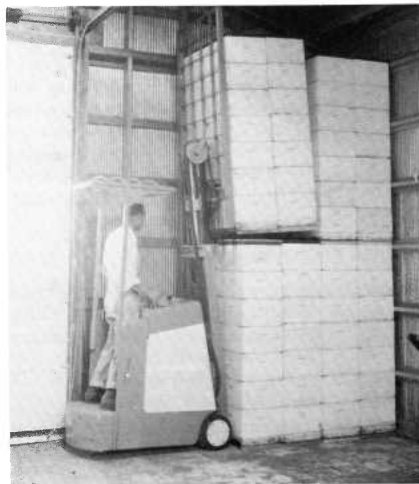
FIGURE 2.—Equipment for moving supers: Top , One-man hand truck with skid board can move several at a time; bottom , power equipment handles many more supers in stacks, as well as drums of honey.
