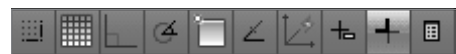
► FIGURE 1.51: AutoCAD 2009: On the Status toolbar, object snaps are displayed as icons.
