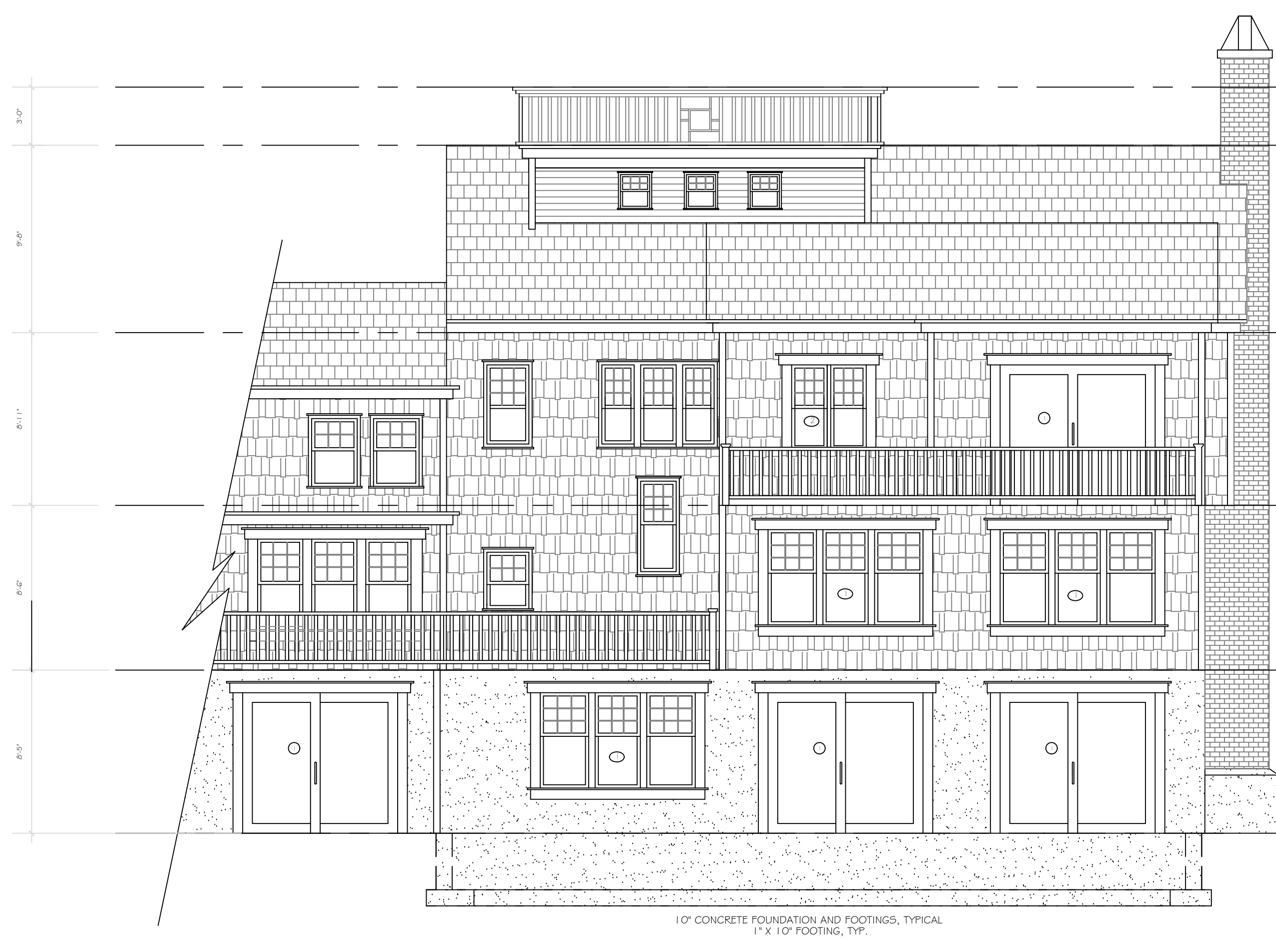
EXTERIOR ELEVATION (NORTH) 1/4" = 1'-0"
