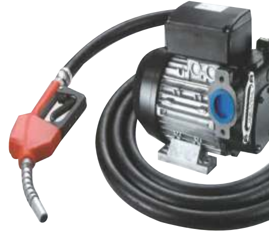
ICT 71900-1 Kit Self priming vein pump for diesel with bypass valve • Flow rate 60L/min • Voltage 220V • Max. Pressure 5Bar • 1" connection ports • Weight 15 Kg • Complete with 4m Discharge Hose & Autoflow • Pack Dimensions 570x430x220
