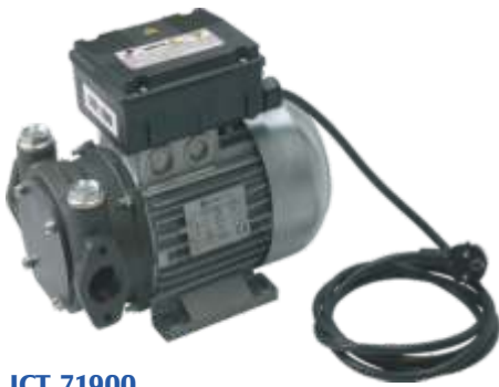
ICT 71900 Self priming vein pump for diesel • Flow rate 70 - 90L/min • Voltage 220V • Max. Pressure 2Bar • 1" connection ports • Weight 9 Kg • Pack Dimensions 290x190x210
