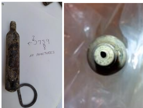
Figure 8 CO 2 Inflation cylinder from Jon's life jacket showing it had not been pierced prior to the incineration
