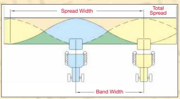
The Teagle Spread Pattern has been developed such that when two adjacent bouts overlap, the graph of total spread is a straight line.
