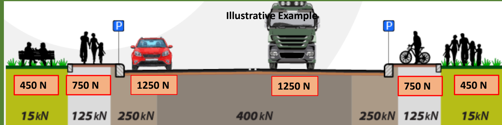
EN 61386-24: Load should not cause internal pipe diameter deformation by more than 5% (limit)
